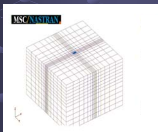
3D Pile-Soil-Pile System
