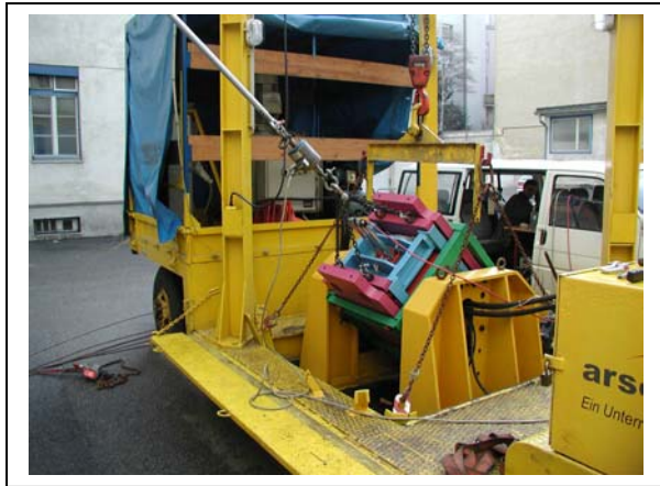
Fig. 2: Insitu test of masonry building Kölblgasse/ Vienna
