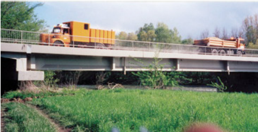
Tests of two trucks on Mura River Bridge (courtesy ZAG, Slovenia)
