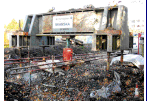
Static load test on 20m long Instrumented 1m diameter bored pile
