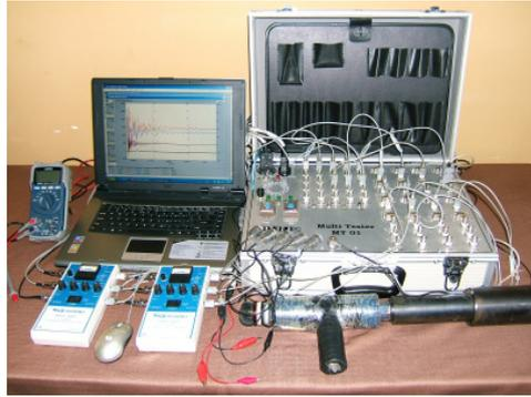
Fig. 1. MultiTester MT01 equipment for seismic qualification of the high voltage electric equipment.
