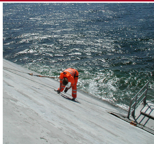
▲ 1.: On-site inspection with Galvapulse equipment
