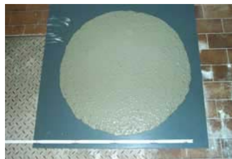
▲ Slump-flow test to evaluate the flow-ability of Self-compacting Concrete
