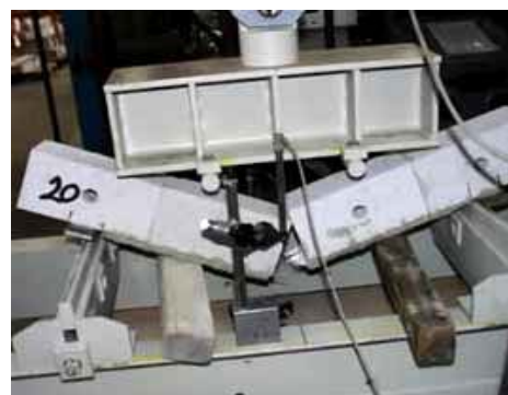
▲ Textile-reinforced masonry test-beam
