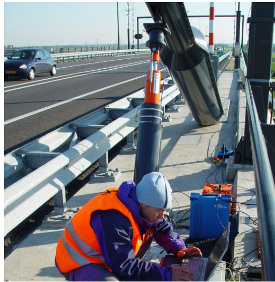
Fig. 73: Taking decay measurements on the “Eiland Bridge” nearby Kampen, The Netherlands.
