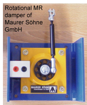
Fig. 52: Rotational MR damper, force range approximately [10, 320] N.
