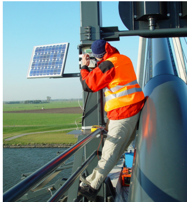
Fig. 84: Solar panel and controller box mounted on the lightning pylon on the “Eiland Bridge” nearby Kampen, The Netherlands.
