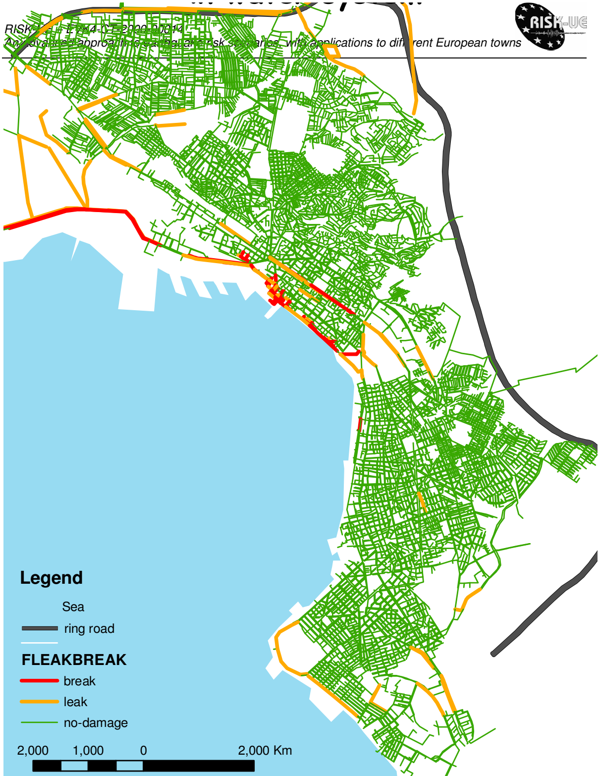
Fig. 6.20 Location of breaks and leaks in the water network of Thessaloniki.
