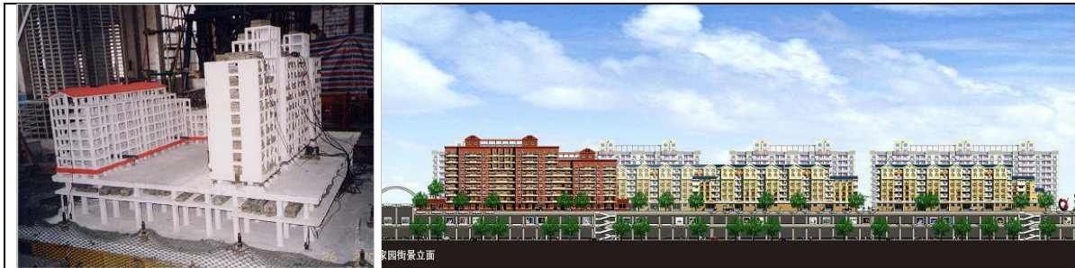
Fig. 6. Mock-up the “Isolation House Building on Subway Hub”, under construction close to the Peking center, which was tested on shake table, and picture of the entire complex.
